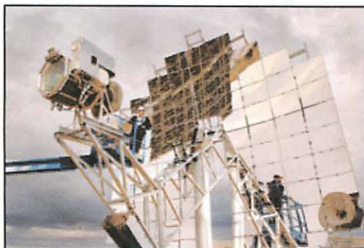
SANDIA RESEARCHER Chuck Andraaka makes adjustments to a Stirling Energy Systems, Inc. solar dish-engine system
