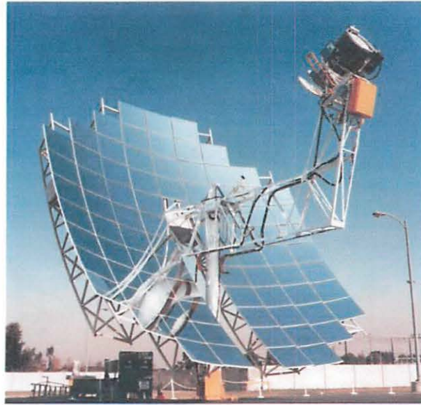
Figure 1.8: Solar Dish-Stirling system. Image courtesy of Stirling Energy Systems (SES).
