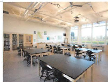
Classrooms at the Kirsch Center for Environmental Studies in Cupertino, California, feature ceiling fans and operable windows to maximize daylighting and natural ventilation.
