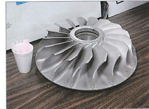
This single-stage, 5-MWe organic Rankine cycle turbine operated on butane at the Mammoth Hot Springs geothermal power plant in California.
