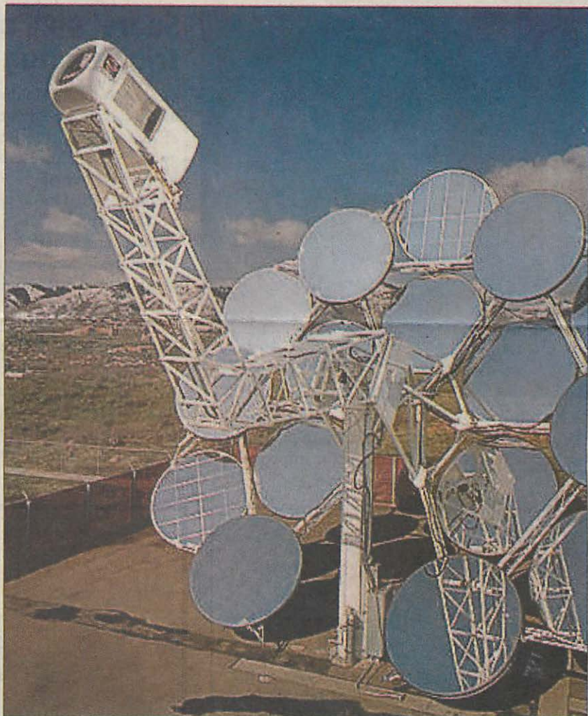
A concentrating-solar-power prototype dish/engine system is in place at the National Renewable Energy Laboratory in Golden. Warren Getz, NREL
