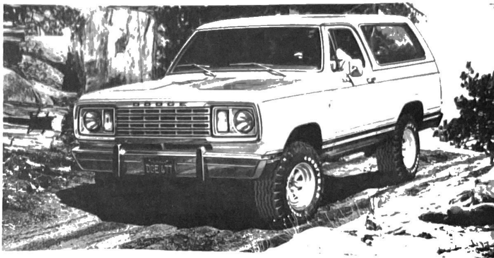
FULL TIME FOUR-WHEEL DRIVE makes this sporty looking 1977 Dodge Ramcharger SE at home on and off the road. Dodge's popular sport utility vehicle is a descendant of the four-wheel drive Dodge trucks that slugged their way through W.W. II. Ramcharger is also available with conventional two-wheel drive.
