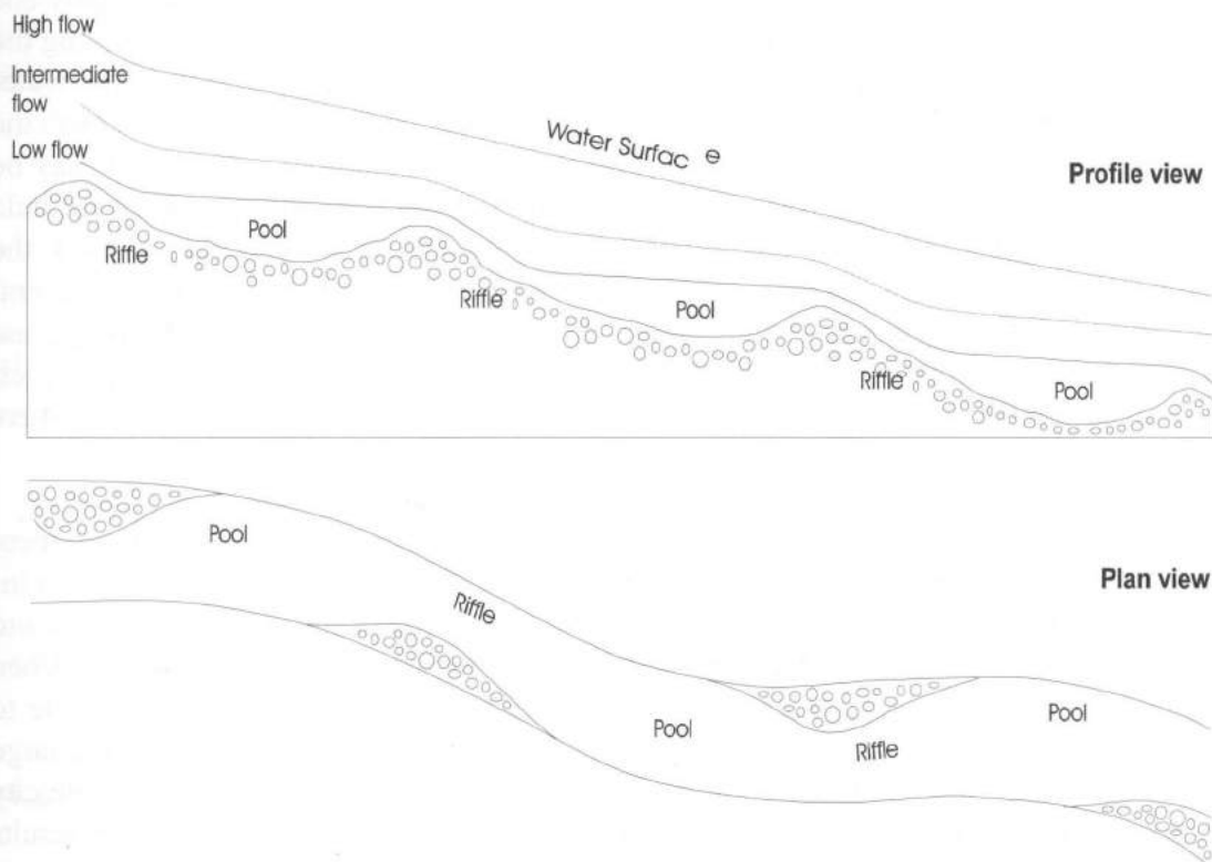
Figure 3.3. Diagram of longitudinal profile and plan view of a pool-riffle sequence. Water surface profiles in upper figure represent high, intermediate and low flow conditions.
