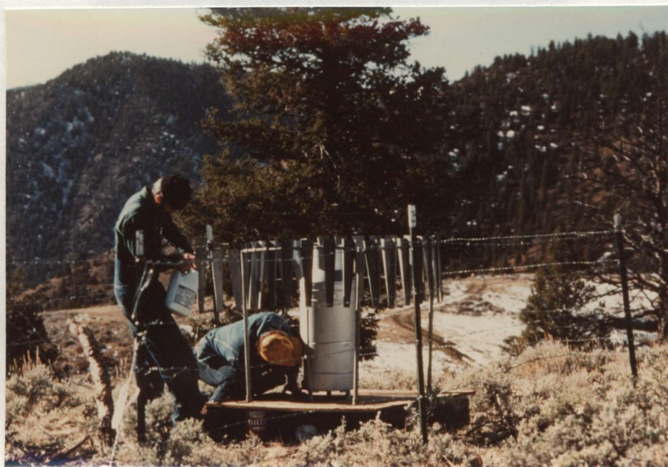
Fig. 6-4. Station 2. Fenced shelter and precipitation gauge.
